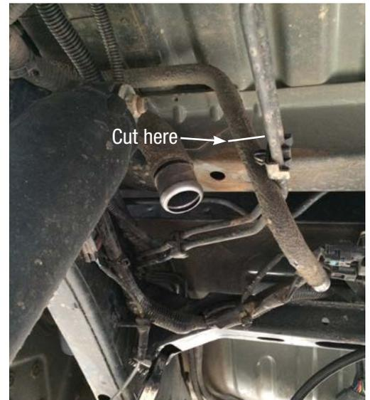
Cut straight piece of fuel filler hose as indicated in image.
