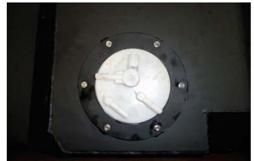
5. Fit tank breather to fuel tank using bolts provided. Carefully remove factory breather hose from fitting at fuel sender. Re-attach breather hose to fuel sender and roll over valve.
