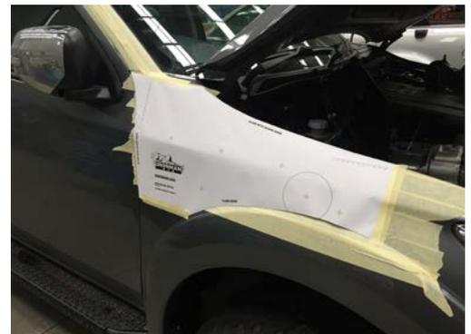
5. Using felt tip pen, mark all holes through template onto mudguard.
