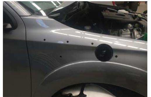
8. Using thread-lock screw all studs into snorkel body and attach pillar mounting bracket loosely to snorkel using M6 bolts provided.
