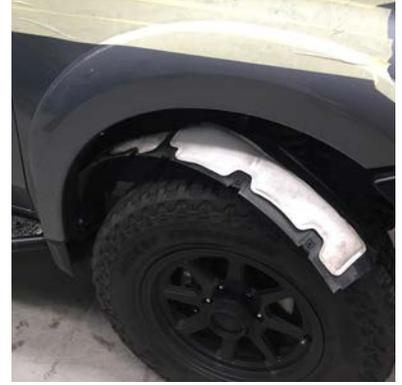
3. Apply masking tape to right hand mudguard and windscreen pillar.
