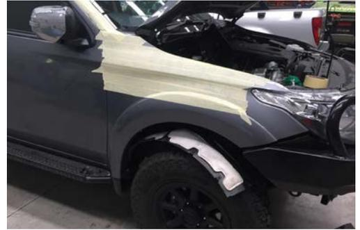
6. Remove template and drill all 5 mounting holes to 12mm (ensure drill does not damage the wiring loom located behind the mudguard). Using a 105mm hole saw cut the remaining hole for the air entry hose.
