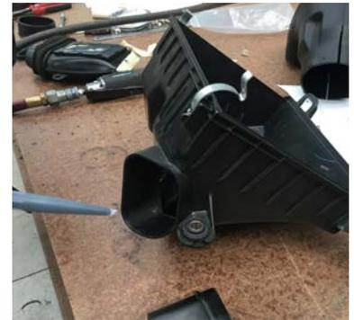
14. Apply sensor safe sealant to the larger side of the air box adaptor and insert into air entry hose and secure with hose clamp provided as shown.
