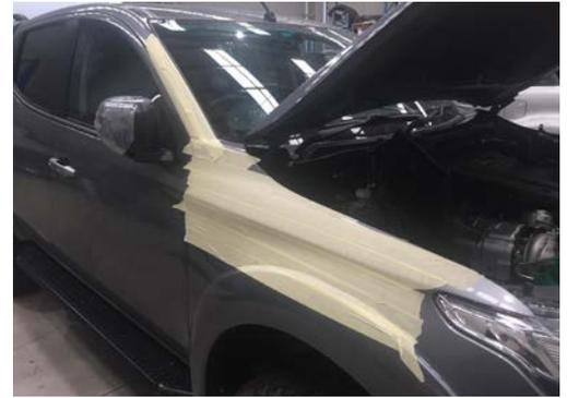
4. Tape template to mudguard making sure it is lined up with the top of the mudguard (bonnet opening), rear of mudguard (door opening) and top of flair.
