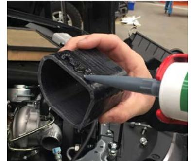
15. Apply sealant to air box intake.
