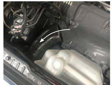
12. Install snorkel body to vehicle using M8 Nylock nuts and body washers provided. Attach pillar bracket using M6 bolts and washers provided. Attach air entry hose to snorkel and secure with hose clamp provided.
