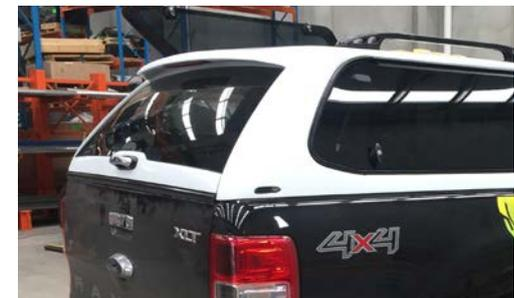
13. Recheck that the canopy is square and aligned evenly with the vehicle tub. Adjust if required.
