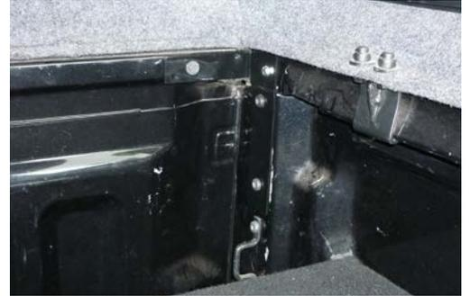
8. Clean top edge of of tub using wax and grease remover.
