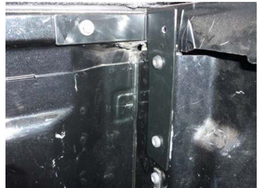
6. Using top hole in bracket as a guide, drill a 6.5mm hole as shown.
