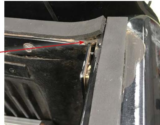
11. Place canopy in position on the tub of the vehicle, being careful not to dislodge the seal.
