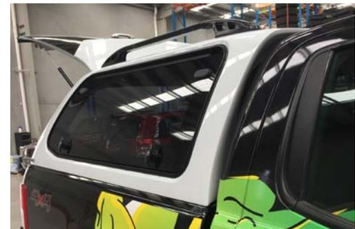
12. Close the vehicle tailgate and adjust the position of the canopy until the rear door closes easily and makes even contact with the tailgate.
