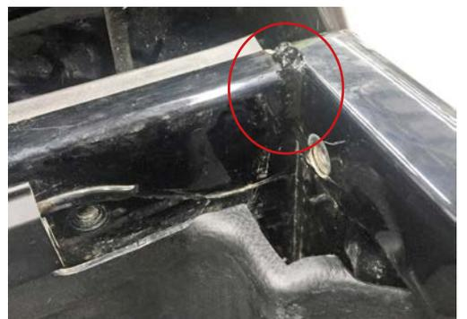
10. Attach adhesive seal to the top of tub and seal all joints with neutral cure silicone.
