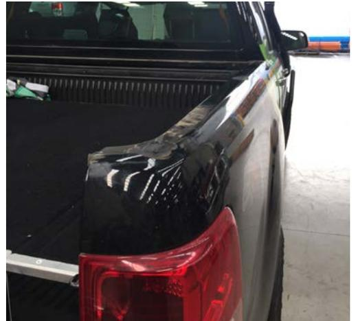
9. Using supplied neutral cure silicone seal any seams or holes that might allow water to enter the tub once canopy is installed.
