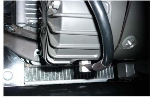
7. Run the positive and negative battery cables into the engine bay taking care to secure cables away from any sharp or moving objects.
