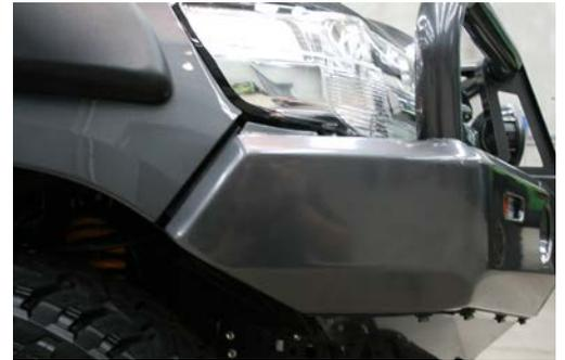
9. Once bull bar is aligned with vehicle and tightened, drill through pinning holes (circled in yellow) between bull bar and chassis bracket and secure the M-10 bolts, washers and nuts provided.
