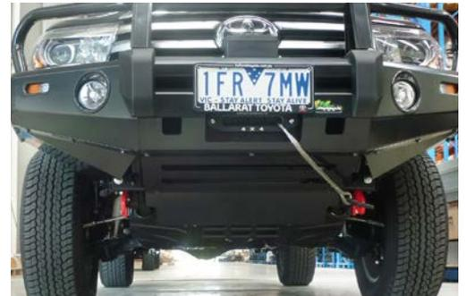
13. Trim guard liners as shown and attach to protection plate using cable ties.
