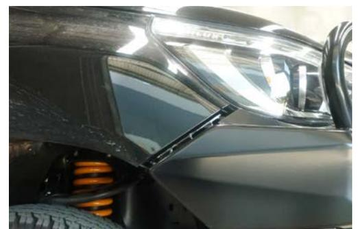
10. Once bull bar is aligned with vehicle and tightened, drill through pinning holes (circled in red) between bull bar and chassis bracket and secure with bolts, washers and nuts provided.
