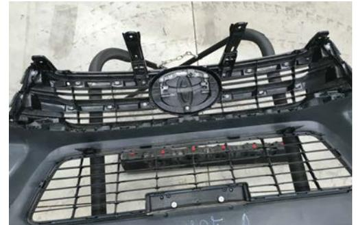
Refit grill using supplied bracket to secure centre section as shown.
