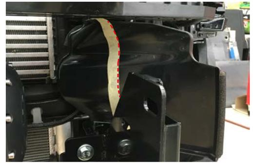
7. Unwrap bull bar. Check over riders and light assemblies are tight in bull bar before installation.
