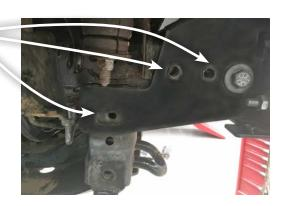
4. Place recovery point into position, and replace the 2 x bolts that pass through the chassis and leave loose.
