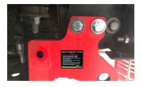
5. Install the 1 x 10.9 bolt and washers provided with the recovery points.
