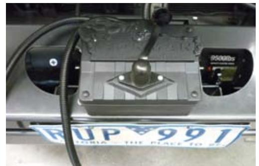
11. Connect three colour coded cables to the corresponding poles on winch motor.
