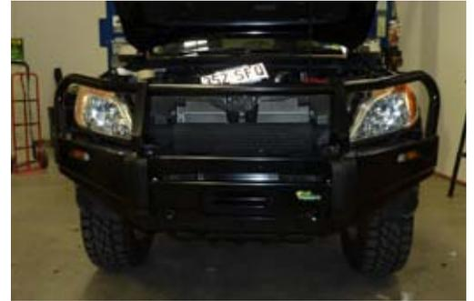
11. Align bull bar with vehicle and tighten all bolts.
