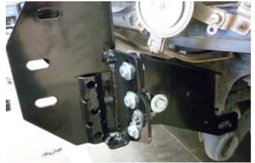
7. Using chassis bracket as a guide, drill a 12.5mm hole through chassis and install bolts, flatwashers, spring washers and nuts as shown,
