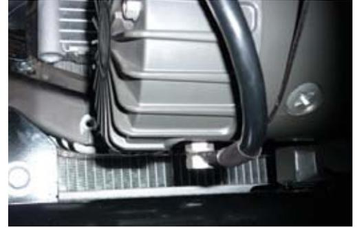
13. Run the positive and negative battery cables into the engine bay taking care to secure cables away from any sharp or moving objects.
