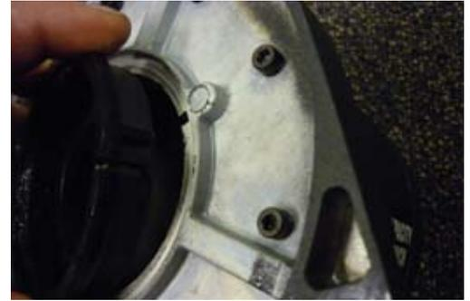
4. Undo and remove 10 Allen head bolts that hold the gearbox housing to the drum support housing and rotate the drum support housing to holes in a clockwise direction so that handle is opposite to the mounting feet.
