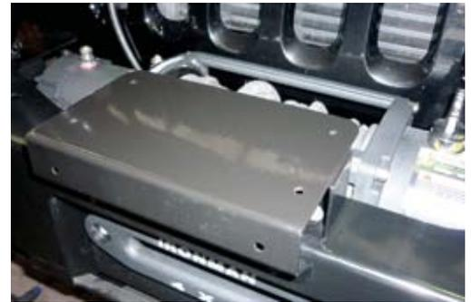
11. Place control box on control box bracket and mark four mounting holes.
