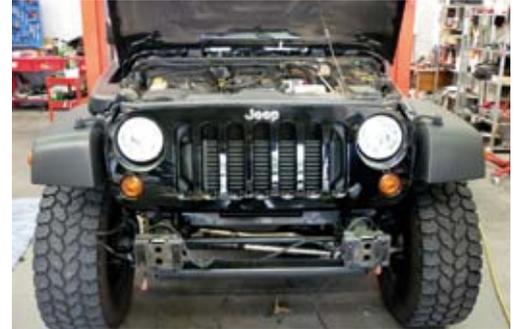
3. Remove fog lights from factory bumper bar and install to bull bar as shown. If winch is being installed, refer to winch installation instructions pages 4-7.
