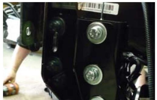
5. Place M12 x 50mm bolts, flat washers and spring washers as shown, through recovery hook on left hand side and packers on right hand side.
