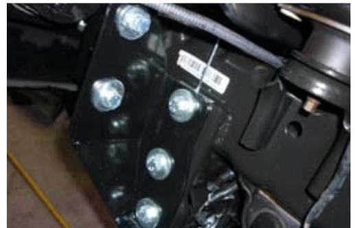
9. Align bull bar with vehicle and tighten all bolts.
